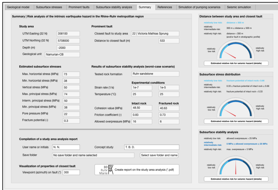
Figure 7: Summary of the most important data for the study area selected by the user in the "Summary" tab. The three geological, experimental, and model evaluation criteria of the potential seismic risk in the study area are shown as risk gauge scales on the right side of the tab.
